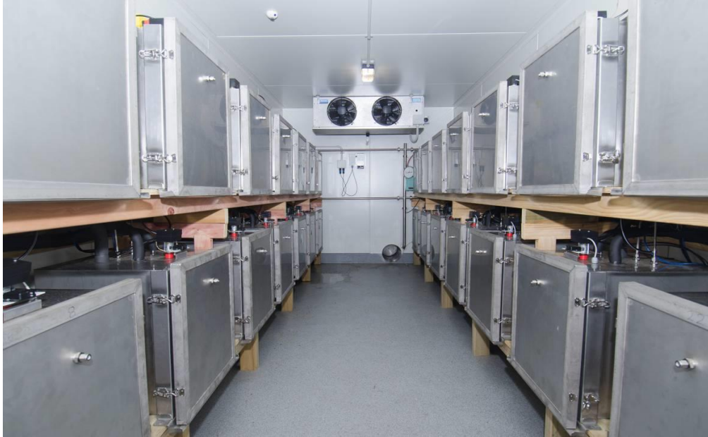
EF treatments facility (78.6-L chambers)
