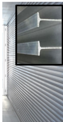
Fig 2: The 'T-bar' floor of a container used to deliver air to the door-end.
